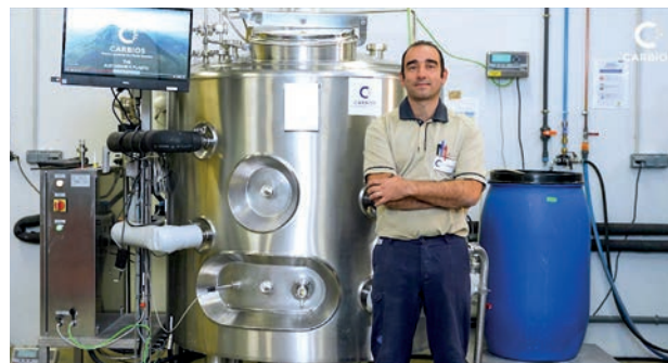
Reactor for the depolymerization of plastic waste and PET textiles into monomers at the Carbios pilot unit.
