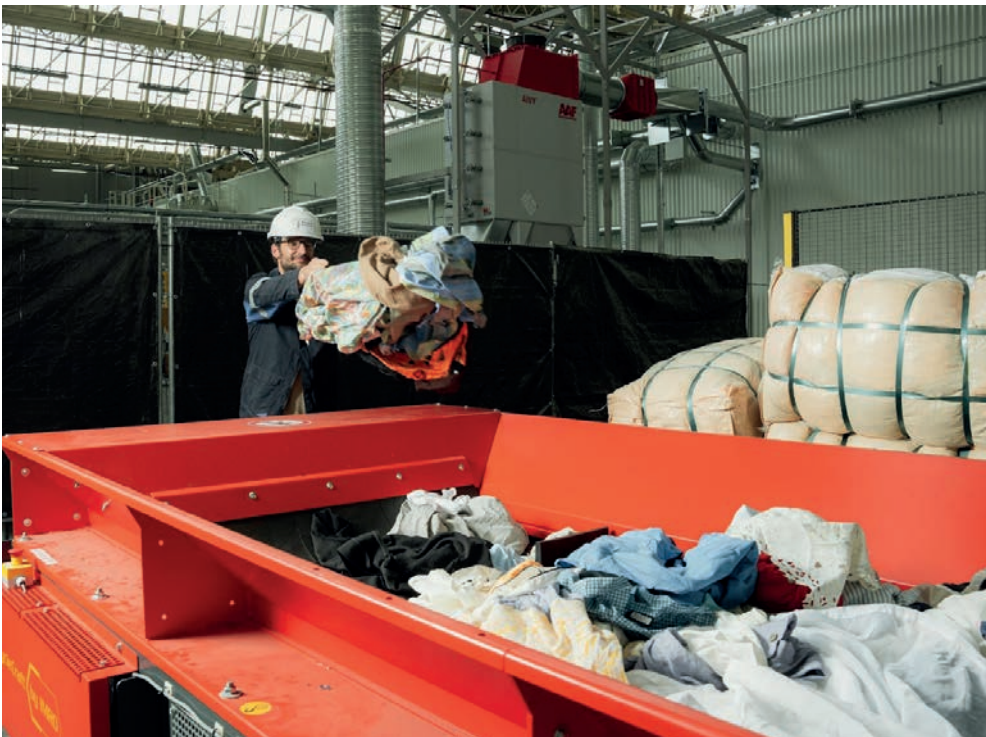
Loading of the demonstration plant's textile waste preparation line. (Carbios)
